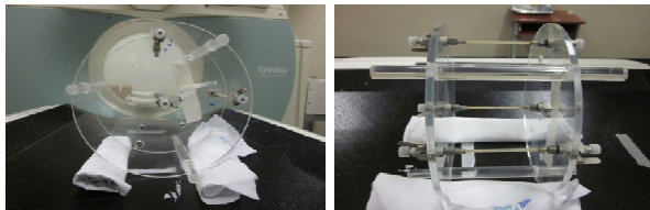
Fig. 2. Insert with 3 linear radiation sources, at the position of air acquisition.
