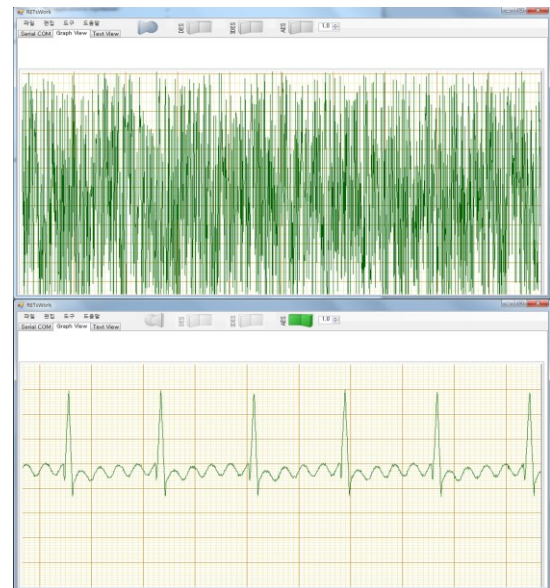
Figure 4. The result of arterial flutter wave: the above noisy waveforms describes the cyphered ECG, and the bottom shows a decrypted ECG waveforms.
