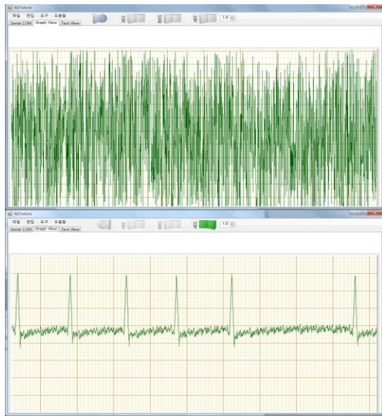
Figure 5. The result of arterial fibrillation wave: the above noisy waveforms describes the cyphered ECG, and the bottom shows a decrypted ECG waveforms.
