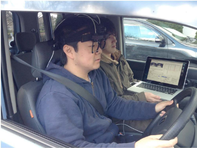
Figure 2. A subject wearing the eye tracker (EyeSeeCam) in the car used in the experiment, and an experimenter holding a PC by which the eye tracker is controlled and all the recording data are stored thru an IEEE 1394 connection.
