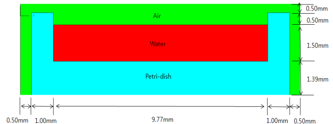
Figure 1. Geometry and size of the culture well considered in the present study. Note that water was taken as the culture medium in the simulation.
