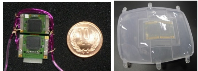
Figure 7. Appearance of the ECoG Measuring Circuits. The right figure shows the location of the circuits inside of the skull case.
