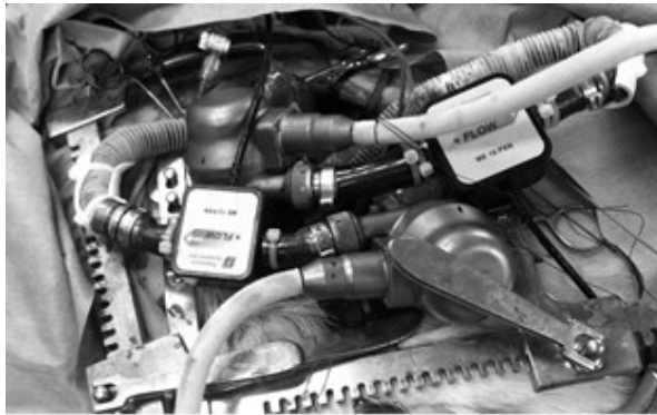
Fig. 9. Overview of the functional total artificial heart circulatory system in animal.
