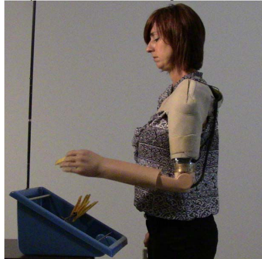
Figure 1. TMR patient with a transhumeral amputation performing clothespin relocation task using the embedded pattern recognition control system.
