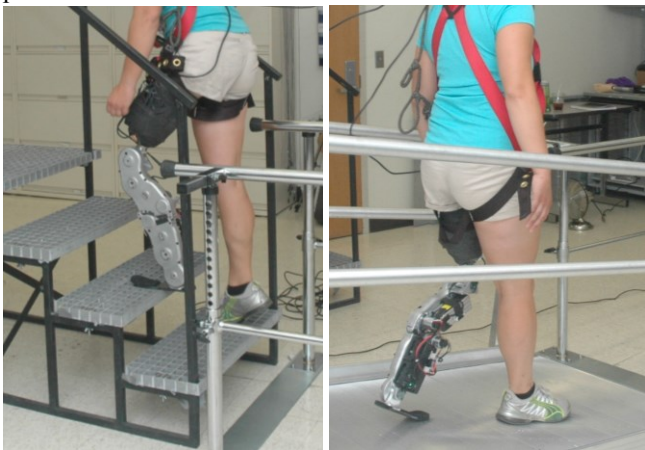
Fig. 1. Transfemoral patient walking on the Vanderbilt powered knee/ankle prosthesis for stair climbing (left) and ramp descent (right).
