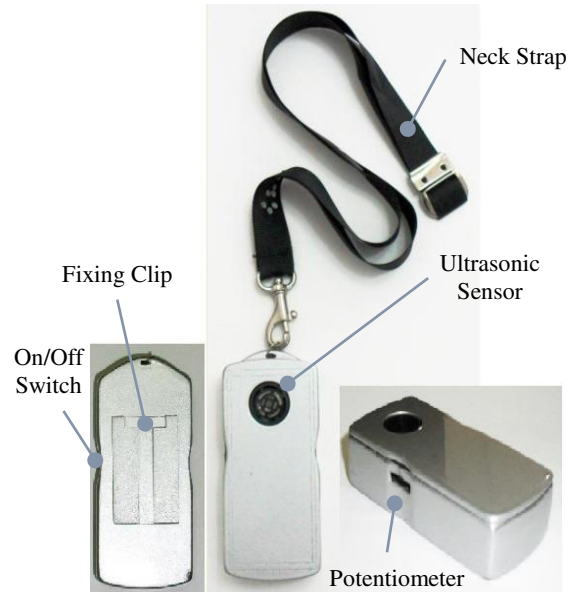
Fig. 3. Fully Packaged Device with Shiny Finish.
