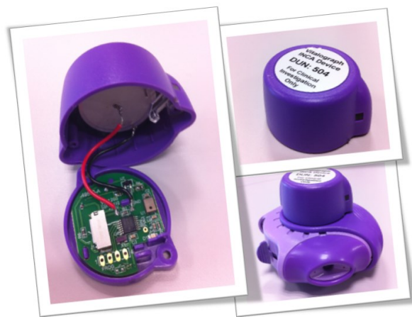
Figure 1: (Left) Internal components of INCA device, (Top Right) External view of INCA device and (Bottom Right) INCA device attached to Diskus™ inhaler.
