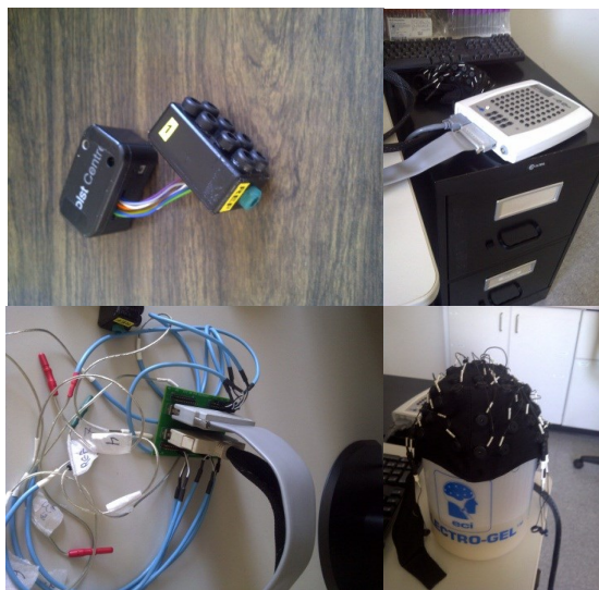
Figure 1: Equipment setup (clockwise from top left) a) Imec 8-channel EEG ASIC; b) NeuroScan SynAmps connection; c) NeuroScan Quik-Cap 64-channel EEG cap; d) Custom-made 80-pin connection board.
