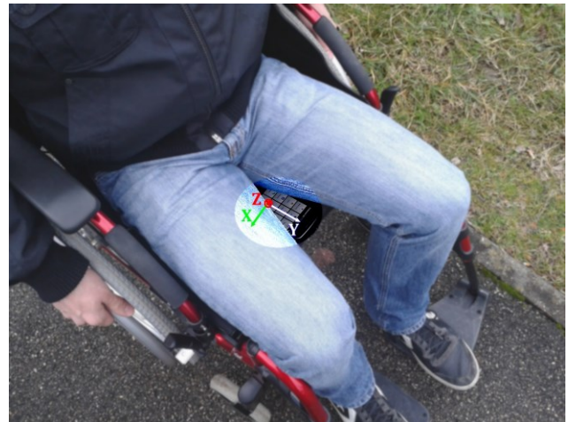
Fig. 3. Smartphone location and acceleration axes.
