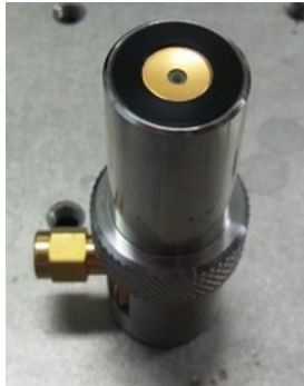
Figure 2. 50-MHz concave transducer with a hole for the optical fiber in the center
