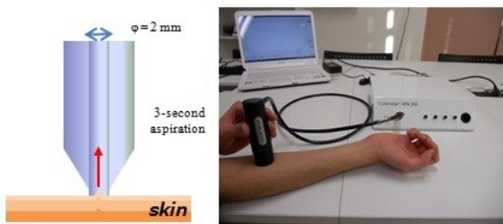
Fig. 2 Principle of measurement system
