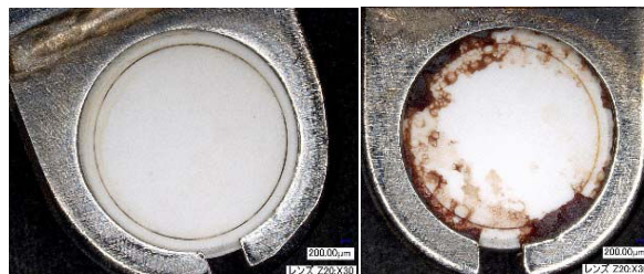
Fig.5 Aspects of RFID tag after cleaning (left: WD group, right: ultrasonic group)
