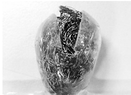
Figure 4. Aneurysm model with stainless steel coils at maximum achievable packing density (PD=15%)
