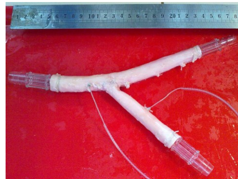
Figure 4. Surgically constructed physical model of arterial bifurcation. The common segment and the two branches are in the same plane, with a bifurcation angle of 60 degrees between branches. Tubing couplers and two Königsberg sensors are shown.
