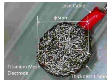
Figure 3 Titanium mesh electrode for the TCS internal unit
