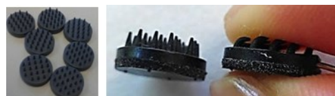
Figure 2. Conductive polymer electrodes using EPDM rubber as matrix combined with conductive additives (such as carbon black).
