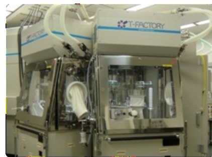
Figure 1. Process of the cell sheet fabrication system [8] (a). Automated cell sheet production system (T-Factory)(b).
