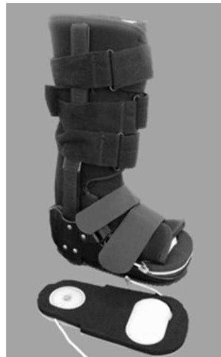
Figure 2. Insole Assembly (IA) component of the LMS both as the insole insert and inserted within a standard CAM walker. In the image of the insole insert the two transducers located under the heel and metatarsal head region are visible.
