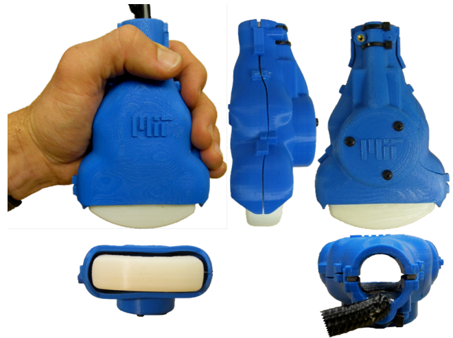
Fig. 1. Front, side, and back views of the six-axis force/torque-measuring ultrasound probe. Depicted with a 3D-printed ultrasound probe mock-up.
