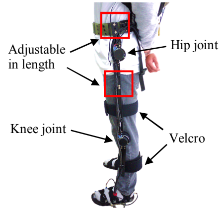
Fig. 2 The designed mechanism for potentiometers. The length of the mechanism is adjustable, and the wires are well integrated into the mechanism.
