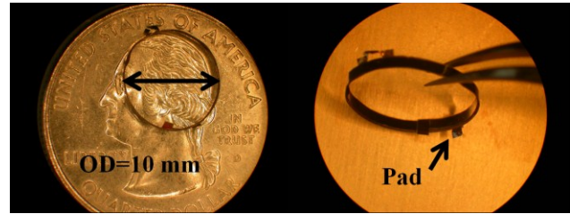
Figure 2. The microfabricated origami foil coil as the receiver coil. The outer diameter is 10 mm.
