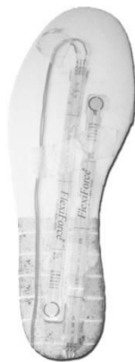
Figure 1: Placement of the two force sensing resistors (FSR) in the insole of the shoe
