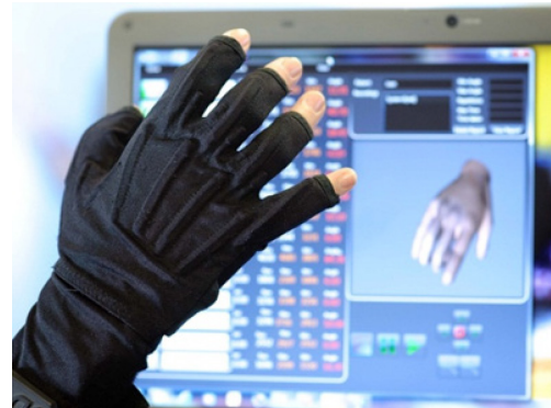
Figure 1. Controlling software with 5DT glove
