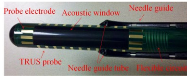
Fig. 2. Probe electrodes plated on the TRUS probe shaft.
