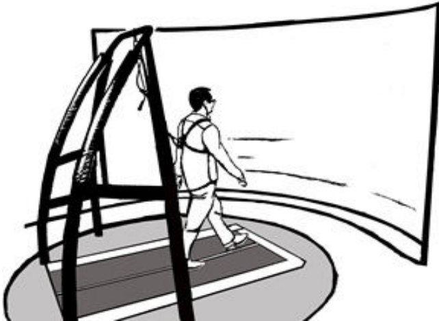
Figure 1: Computer Assisted Rehabilitation Environment (CAREN). A subject walks on the integrated treadmill while facing the synchronized projection screen. In the event of a stumble or fall, the subject is harnessed and tethered to a safety system.
