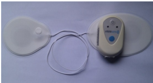
Figure 5: The Aingeal device with impedance based electrodes that detect both ECG and respiration signals
