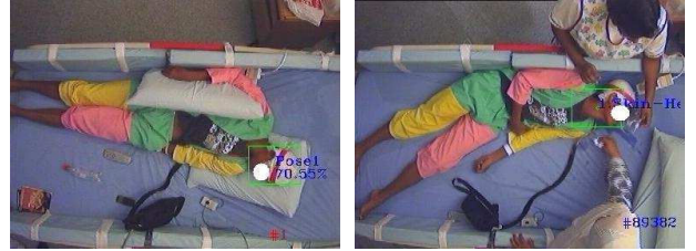
Fig. 5. Left at start, Right after 2 hours. Sample patient's detected face/head. The box shows the detected face/head with various poses and confidence levels (%).
