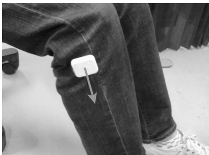
Figure 3. Wireless acceleration sensor used for the evaluation of pedaling balance between the right and left feet
