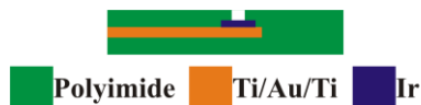
Figure 2. Cross-sectional view of the polyimide neural probe with 1 layer of trace metal. (Images are not drawn to scale.)
