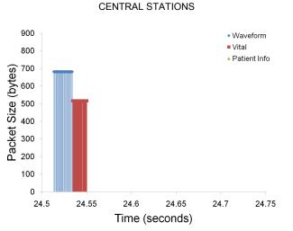
When we configured one bedside monitor to communicate with 35 central stations, we found that the bedside monitor conducted redundant communications with each central station. Here, we show a single 250 ms interval, noting that the bedside monitor output 35 packets with waveform data to the 35 central stations, as well as 35 packets with numeric vital sign values, all within a fraction of the 250 ms interval.
