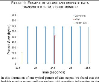
bedside monitor output uniform packets with waveform information to the central station every 250 ms. Numeric vital sign values and patient identification information was transmitted in separate packets sent less frequently, as illustrated.
