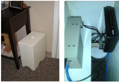
Figure 1 Radar unit placed in a non-hazardous position (left). The radar, DAQ and wireless inside of the box
