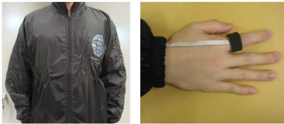
Fig. 2. Outlook of the wearable system in the form of a shirt. Left: electrodes and circuits knitted inside the shirt. Right: Flexible finger-ring sensor as an extension of the shirt.
