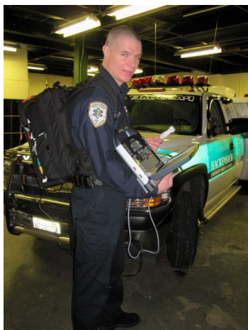
Figure 1- The portable system consists of a LiveU Transmission equipment backpack with Sonosite portable ultrasound machine.
