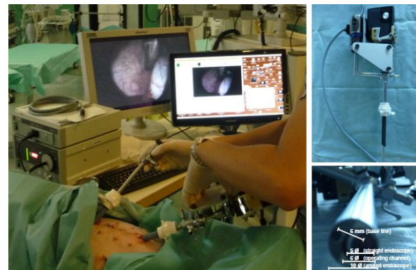
Fig. 8: (left) The 3-D laparoscope in the operating room at IRCAD France. (top right) The laparoscope with coded structured light (SubPerfect map) and a video projector (in black) for epipolar-based patterns. (bottom right) Details of the operating channels at the tip of the instrument: the base line is 6 mm for this 10 mm laparoscope.
