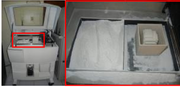
Figure 3. The mold printed in a 3D printer.
