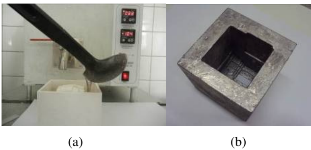
Figure 4. (a) Filling the mold with a liquid cerrobend alloy. (b) The final IMRT compensator block
