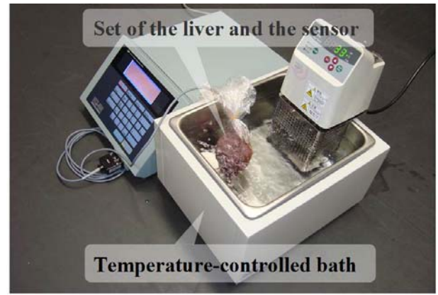
Fig. 1 Experimental setup using a temperature-controlled bath
