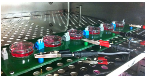
Fig. 1. Detail of the electrical stimulation setup inside the cell culture incubator: the Printed Circuit Board (PCB), cultures plates and inserts including the stimulation electrodes. See text for details.
