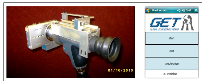
Fig. 1. The camera-ophthalmoscope attachment (left) and a screen shot of the mobile phone application (right)
