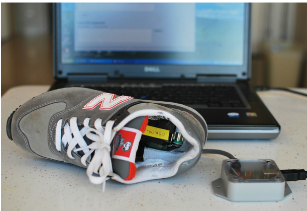
Figure 1. The ActiveGait System. The picture shows the instrumented shoe together with the connections and software component of the system.
