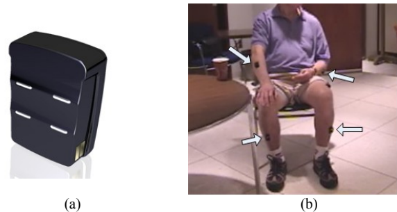
Fig. 1. (a) One of the wireless sensors used by our system. The sensor collects three channels of data from a triaxial accelerometer and one channel of surface electromyographic data. (b) A PD patient wearing one sensor on each limb (as indicated by the arrows) during testing in an apartment-like setting.
