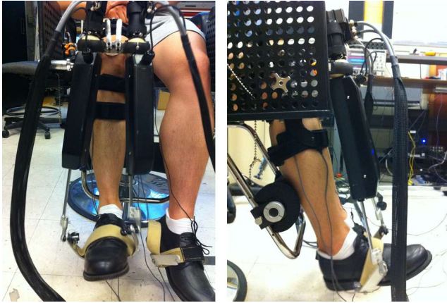
Fig.1. A subject wearing the Anklebot in a seated posture (left: front view, right: side view)
