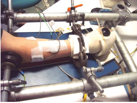
Fig. 1. Experimental setup. The hand and distal part of the lower arm are fixated. A robotic manipulator provides short angular deviations around the wrist.
