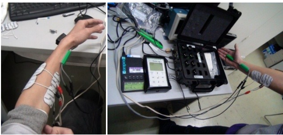
Fig. 5 Sensors and FES electrodes on the subject for tremor generation.
