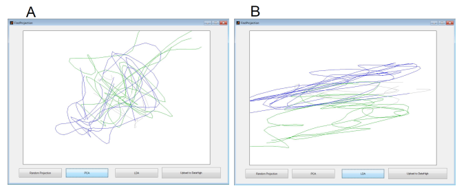
Fig. 3. Static 2D projections found by standard methods, A: PCA and B: LDA, when applied to the data shown in Fig. 1. In contrast, DataHigh (Fig. 1) can find a dynamic 2D projection in which the trajectories splay out over time and are largely non-overlapping for different reach conditions.
