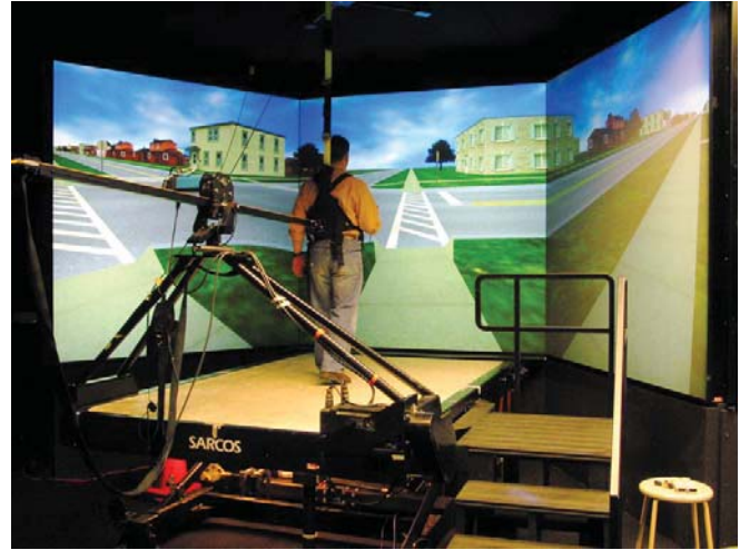
Fig. 1: Treadport virtual environment comprising a CAVE-like visual display and locomotion interface. This image, shown for clarity, was taken before the addition of the active wind tunnel and Vicon motion capturing system.
