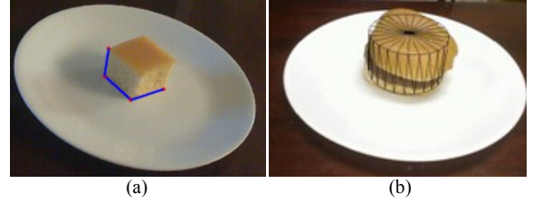
Fig. 3. The measurement of geometric dimensions in images. (a) ‘‘point-clicking’’ method; (b) ‘‘wireframe-fitting’’ method.
