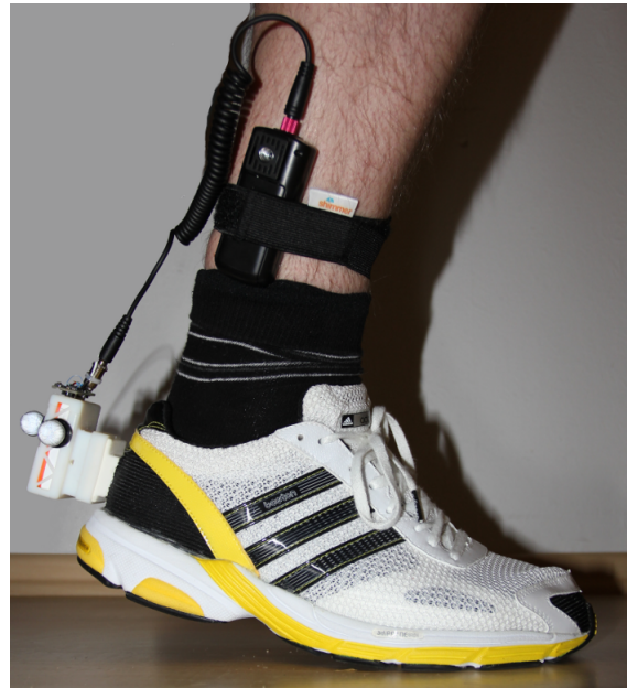
Fig. 2. Setup for synchronous kinematic recording. A Shimmer node was mounted to the heel of a running shoe and connected to a trigger receiver fixed at the ankle. Three reflective markers were added for evaluation.
