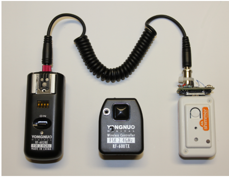
Fig. 1. The main components of the wireless system: trigger receiver (left), trigger transmitter (middle) and modified Shimmer sensor node (right).
